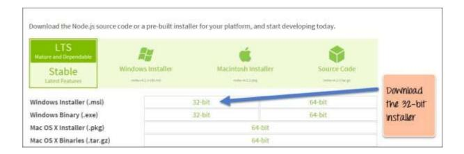
**Step 2)** Double click on the downloaded .msi file to start the installation. Click the Run button in the first screen to begin the installation.
